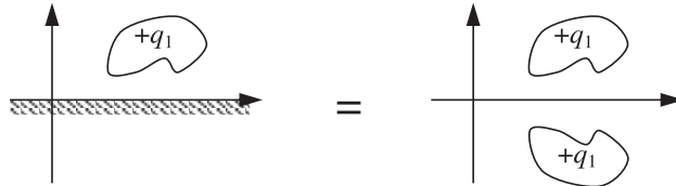
FIGURE 6.15 Illustration of the method of images for the flow generated by a source distribution near a horizontal wall. An image distribution of equal strength mimics the effect of the solid wall.
