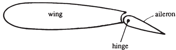
FIGURE 13.4 The aileron. As shown, this aileron deflection would increase lift by increasing the camber of the effective foil shape.
